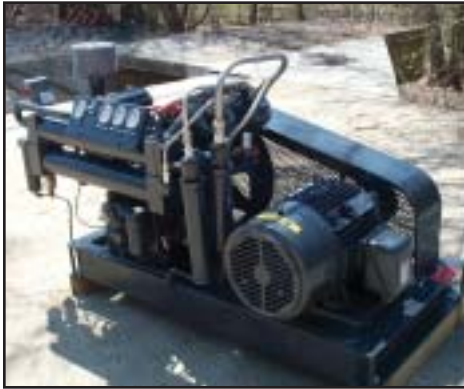
■ A 20 year old Williams & James compressor overhauled and upgraded by GAS in April, 2003. Application: Breathing Air, Discharge Pressure: 3000 psig (204.12 bar).
