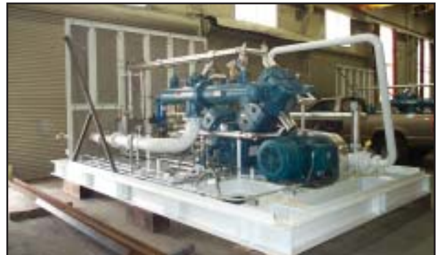
■ One of three process oxygen compressor packages completed by GAS in 2003. The package incorporates a Belliss & Morcom Model V-130 compressor and is used to raise the pressure of oxygen produced in a VPSA or cryogenic oxygen generator.
