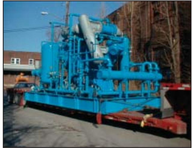
■ Oil-free reciprocating compressor package delivered by GAS in 2000, incorporating a Belliss & Morcom 3-stage model W1100. Application: Nitrogen boosting from a cryogenic plant to 500 psig (34 bar) for slag treatment at a steel mill.
