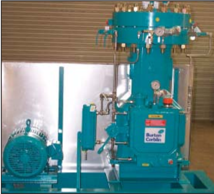
■ A diaphragm compressor package completed by Gas & Air Systems Inc. (GAS) in January 2003. The package incorporates a Burton Corblin Model D123LC6.3 metal diaphragm compressor. It is used to compress high purity nitrogen gas to a pressure of 900 psi (61.2 bar) with zero contamination of the gas.
